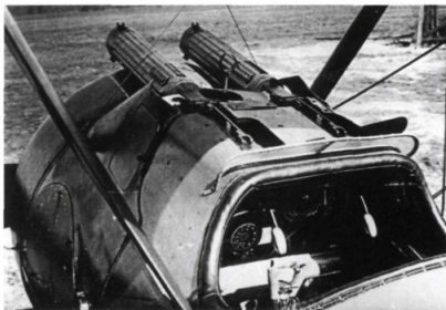
A view of a Sopwith Camel cockpit. The amount, and placement, of instrumentation was not uniform, and the presence of a 'blip switch' on the control column depended on whether the aeroplane had a Le Rhône or Gnome engine. Pilots of Bentley BR 1-powered Camels operated a throttle. [Philip Jarrett]
