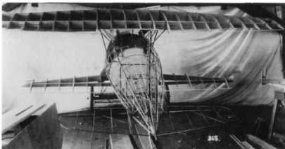
A stripped-down V 1 displays the innovative wooden box cantilever wing structure that Anthony Fokker adopted because it was lighter than Dr Hugo Junkers' all-metal configuration – as well as the sesquiplane configuration he had had in mind before the Idflieg insisted upon a triplane layout. [Museum of Flight Peter Bowers Collection]
